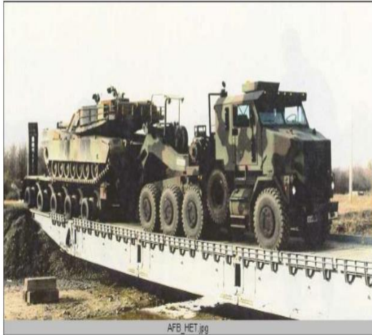
Combined wheeled vehicle: US Heavy Equipment Transport System (Tractor M 1070 + semi-trailer M 1000)
